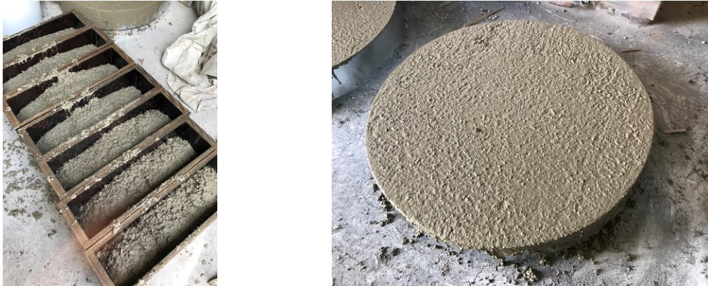
Fig. 2. Specimens during preparation according to EN14651 and SIA 162/6
